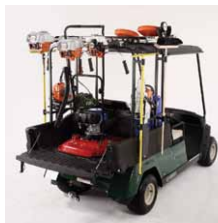
The front and rear views of the Yamaha YTF2 utility car fitted with the locally designed tool-carrier rack, keeping your STIHL brushcutters/edgers and chainsaws safe and secure.
